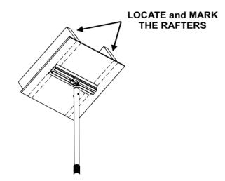
**Installer Note:** The Ceiling Channels are pre-drilled at 16 inch centers. If the spacing on your joists is different you will need to drill new holes in the Ceiling Channel to suit.
